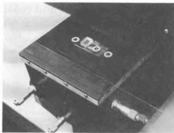
FIG. 1. A picture of the liver specimen placement on the stage of the SLAM. The inside and outside diameters of the metal spacers are 6.4 and 13 mm, respectively.
