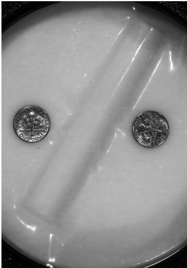
Figure 2. Reference phantom surface revealing the slot in which the transvaginal transducer probe was positioned to obtain a full-field B-mode image (as well as the raw radiofrequency data). Scale: U.S. coin (dime) has a diameter of 1.8 cm.
