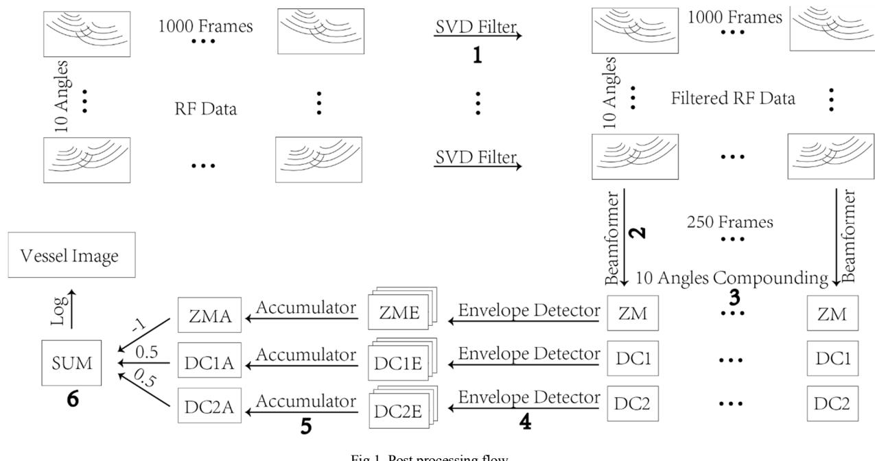
Fig.1 Post processing flow
