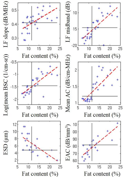
Fig. 1. LF (slope and midband), QUS (mean BSC and mean AC) and QUS-derived (ESD and EAC) parameters as a function of fat percentage for *ex vivo* conditions. The red dashed lines correspond to the best linear fits. The black lines correspond to a fat percentage threshold of 11.6 % and to LF, QUS and QUS-derived thresholds defined to separate normal from fatty livers.
