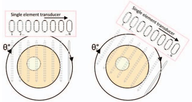
Fig. 2. Proposed full angular spatial compounding configuration. A single element transducer is moved laterally to create an N multi-linear data sample of the target. Process is repeated over a full angular stepped trajectory of 360°
