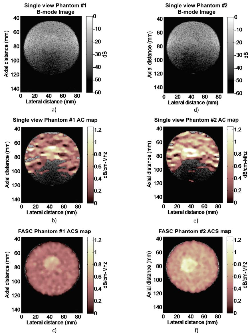
Fig. 3. (a),(d), Examples of the B-mode images obtained from single view of both phantoms. (b),(e), Corresponding single view attenuation coefficient images. (c),(f) Full angular spatial compounding attenuation maps for both phantoms.
