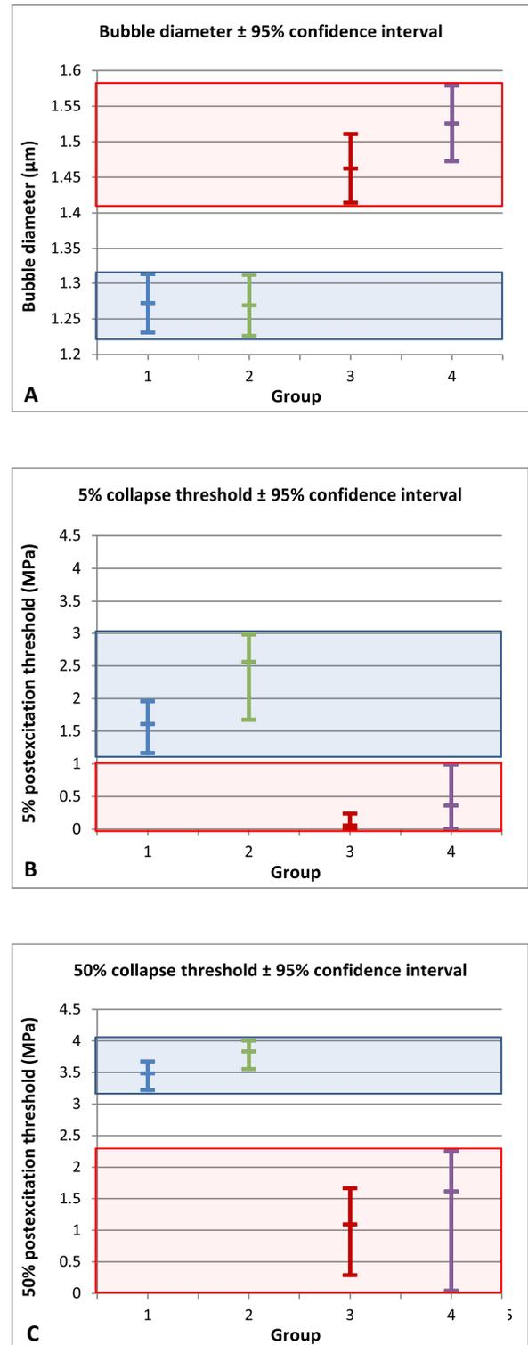
Fig. 2: Plot of 95% confidence intervals for the determined mean bubble diameters (A), 5% (B) and 50% (C) collapse thresholds for the 4 tested groups
