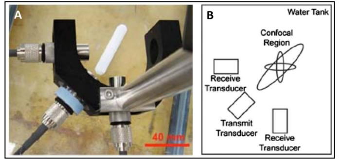
Fig. 1: (A) Photograph and (B) schematic of the DPCD experiments as described by King *et al* [14]
