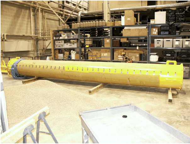
Fig. 1. Impedance tube in the horizontal position, showing the microphone ports. Photo by Timothy Onder.
