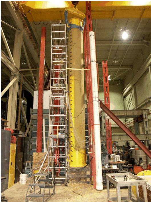
Fig. 2. Impedance tube in the vertical position. Microphones not installed. Photo by Timothy Onder.
