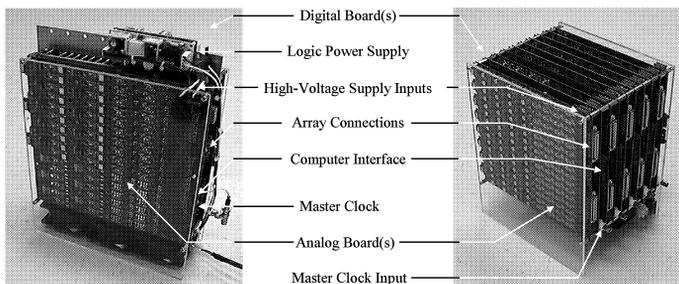
**FIGURE 7.** 20 Channel High-Power System (left) and 320 Channel Low-Power System (right).
