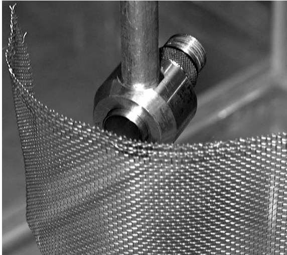
Figure 5: Experimental set-up showing transducer and wire mesh phantom.
