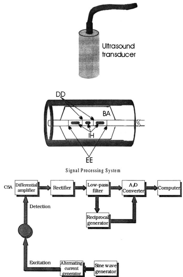
**Fig 1.** Top: Schematic drawing of the impedance planimetry probe and the ultrasound transducer. The excitation and detection electrodes are denoted by EE and DD, respectively. IH indicates side-holes connected to a fluid container for pressurizing the balloon (BA). Bottom: Block diagram over the impedance planimetry signal processing system.
