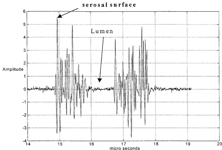
**Fig 2.** A-scan pulse-echo ultrasonic signal showing the esophageal wall with its serosal and luminal surfaces.
