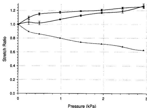
**Fig 4.** Illustration of stretch ratio in circumferential (◆), longitudinal (▼), and radial (▲) direction as function of the distension pressure. See text for definition of stretch ratio. Incompressibility was assumed. The balloon distension caused axial elongation to a lesser degree than the circumferential stretch.
