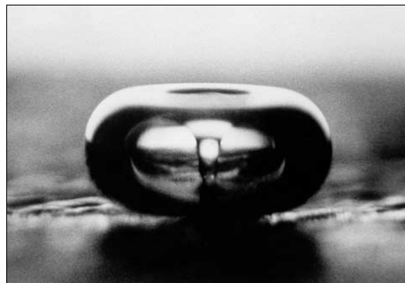
Figure 4-1 Collapsing bubble near a boundary. When cavitation is produced near boundaries, a liquid jet may form through the center of a bubble and strike the boundary surface. (Photo courtesy of Lawrence A. Crum, PhD.)
