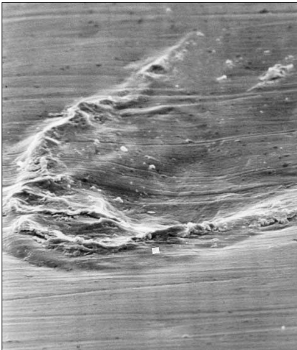
Figure 4-2 Pitting caused by cavitation on a brass plate due to exposure to a lithotripter. (Photo courtesy of Lawrence A. Crum, PhD.)
