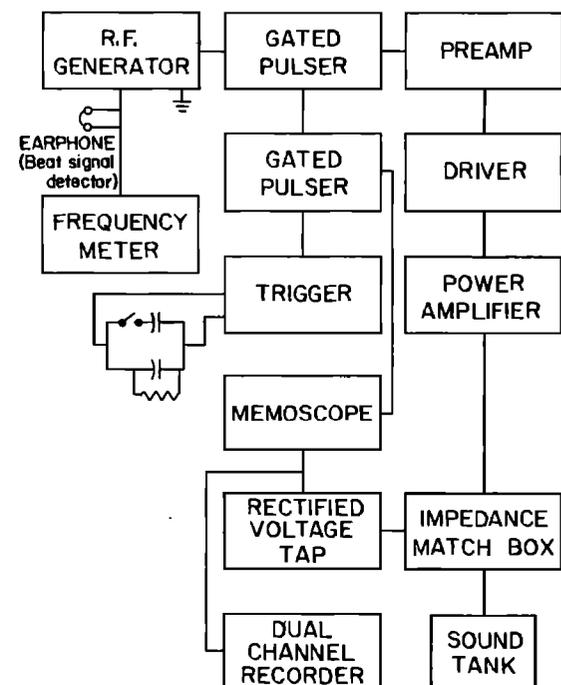
FIG. 2. Block diagram of ultrasonic generation and control instrumentation.
