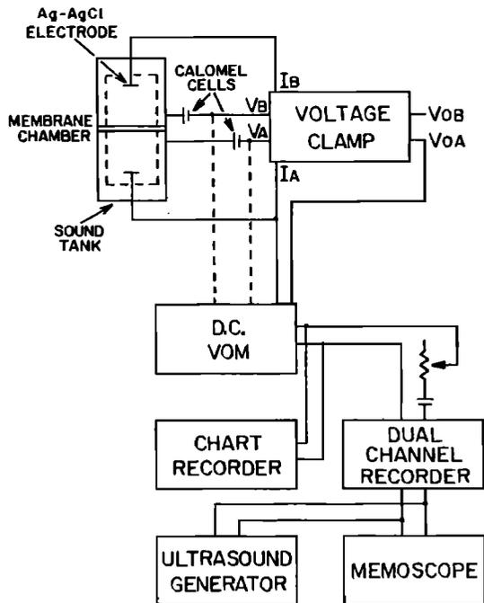
FIG. 1. Block diagram of electrical measuring and recording instrumentation.
