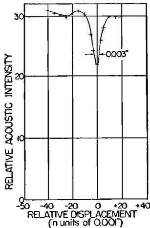
FIG. 2. The detection of the presence in the coupling liquid of a 0.003-in. nylon filament by the ultrasonic microscope operating at a frequency of 12 mc/sec.
