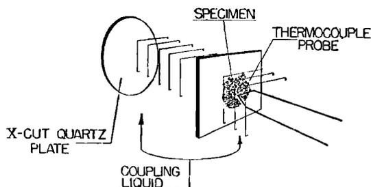
FIG. 1. Schematic representation of ultrasonic microscope showing transducer plate which is excited to produce pulses of ultrasound in the coupling liquid, the specimen under examination which is movable in the coupling liquid, and the thermocouple probe whose junction is placed immediately adjacent to the specimen.
