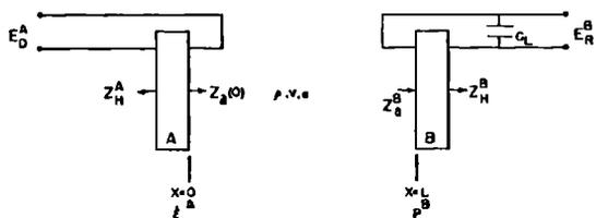
FIG. 5. Schematic diagram of crystals and terminations. The quantities  $\rho$ ,  $V$ ,  $\alpha$  are the density, acoustic velocity, and absorption coefficient per wave-length of the coupling medium.
