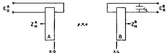
FIG. 1. Schematic diagram of crystal geometry with both electrical and mechanical terminating impedances indicated.
