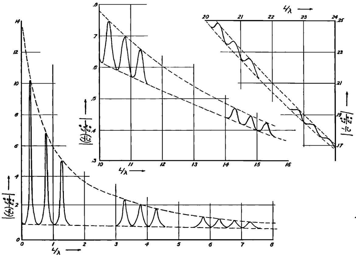
FIG. 6. Typical curve of the ratio of receiver voltage to driver voltage as a function of the crystal spacing in wave-lengths for a highly absorbing medium.
