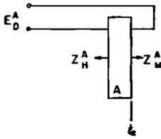
FIG. 2. Driver crystal and terminations.
