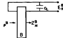
FIG. 4. Receiver crystal with acoustic driving pressure and voltage generated across a capacitive load indicated.
