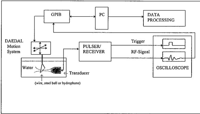
Fig. 1. Block diagram of the main system components.
