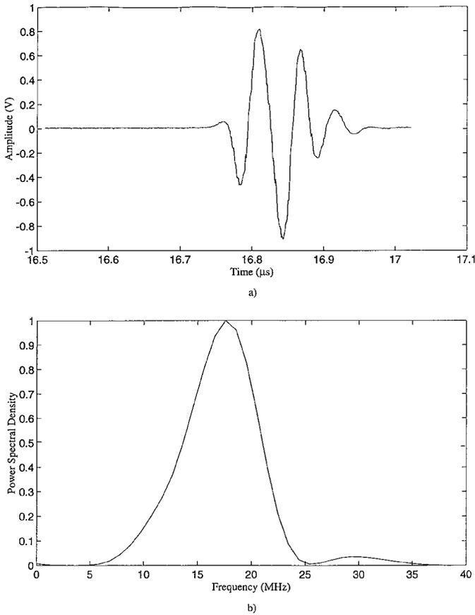
Fig. 2. (a) Pulse-echo response and (b) power density spectrum of the 20-MHz transducer field. A 25- $\mu\text{m}$  wire target was positioned at the on-axis true focal location.
