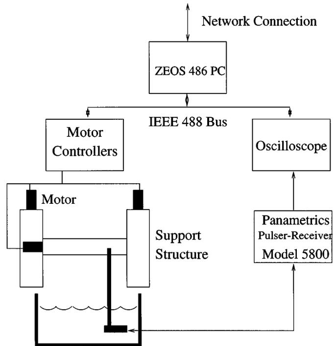
Fig. 3. Schematic of data collection system.
