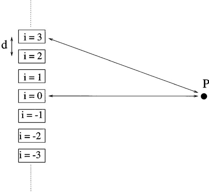
Fig. 1. Geometry of focusing situation. Elements are numbered such that the zeroth element is the center element of the subaperture.  $P$  is the desired focal point and  $d$  is the interelement distance.
