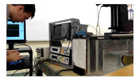
Use the trigger out from the transmitting source as the trigger sync for the hydrophone's received input signals.
