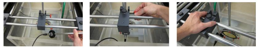
A. Secure the metal rod with the transducer to the sliding clamp on the rail above the Daedal tank. Make sure to align the face of the transducer with the ring. They must be parallel. If they are not parallel it will be impossible to find symmetry around the focus.
