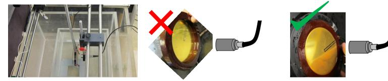
The flat gold side of the Hydrophone, must face the transducer.
