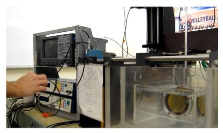
Use the cable which came in the hydrophone case to connect the output of pre-amp to the input channel of the daedal.
