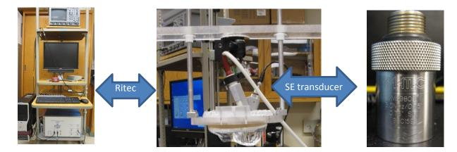
Many BRL experiments use a single element transducer with the Ritec system, as illustrated in the upper middle photo. It is usually desired to know the spatial pressure levels produced from an ultrasound device for the experimental design. Therefore, a calibration is performed. BRL SE transducers are designed to transmit through biological tissue. Since tissue is mainly comprised of water, the SE transducer are impedance matched to water and calibrations are done in water.
