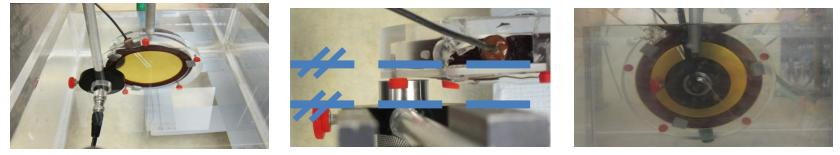
B. Slide the transducer to an edge of the hydrophone. Rotate the transducer to make sure it is parallel with the hydrophone. The transducer should be approximately centered along axis three in reference to the hydrophone and over the active element.
