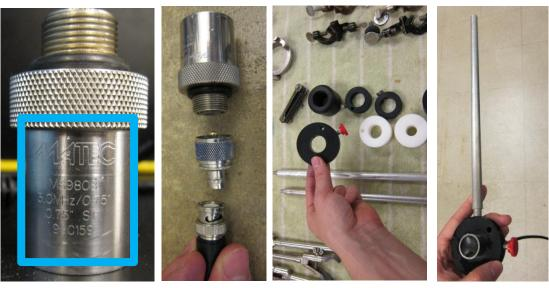
A. Record the transducer B. Attach the properties. Write down the serial number, model number, frequency and f number (focal length/diameter) of the transducer as well as the date of the scan.
