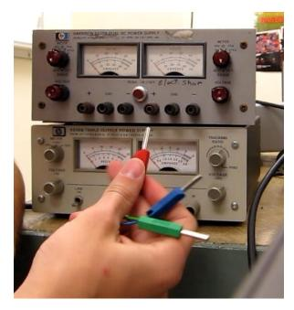
The matched pre-amplifier is used with the hydrophone when performing calibrations. Its multicolored plugs must be connected to a power supply. There are two power supplies located next to Daedal 2 on the table behind the computer. Either one can be used; however, the bottom power supply is preferred. The proper color plug to port connections are stated on the pre-amp.
