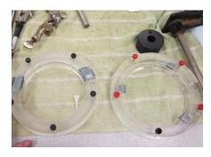
The hydrophone holders are located on the accessory table in the daedal room. There are two hydrophone holders that can fit the Marconi hydrophones. Remove the holder ring piece with the thumbscrews. Remove the hydrophone from the case by only touching the wooden edges.
