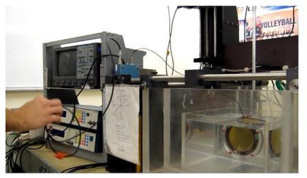
Use the cable which came in the hydrophone case to connect the output of pre-amp to the input channel of a monitoring device.
