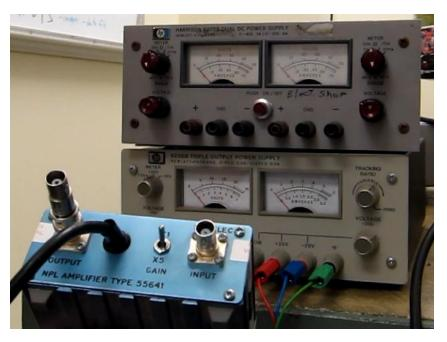
Simply plug the red plug into the +20 v port, the blue plug into the -20 V port, and the green plug into the GND port.
