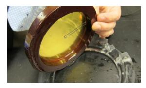
Place the concave part of the hydrophone face down in the thick holder piece. The hydrophone is very fragile and must be handled with extreme care. Do not touch or wipe the face of the hydrophone (let air dry).
