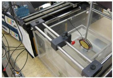
Put the hydrophone in degassed water; all of the gold membrane must be submerged. Once it is completely submerged connect the cord from the hydrophone to the input of the pre-amp.
