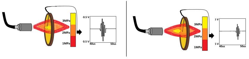
The hydrophone is used as the receiver for transducers in thru-transmission mode to measure material insertion-loss, attenuation, and speed of sound.
