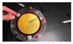
Secure the hydrophone in the holder by tightening the thumb screws finger tight. Screw in a rod (at least 24" inches) in the right threaded hole on the edge of the holder.
