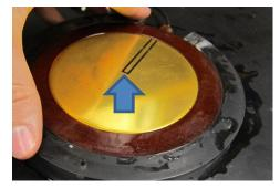
The flat side of the hydrophone must sit face up in the holder. The hydrophone is directional. The Hydrophone's active element is calibrated to this face direction. The transmitting source must be in placed in front of this face.
