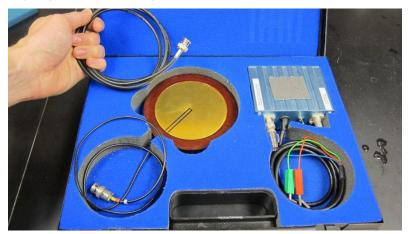
Each hydrophone is stored in a protective case; it comes with a matched pre-amplifier and cable that must always be used between the pre-amp output and monitoring scope input.
