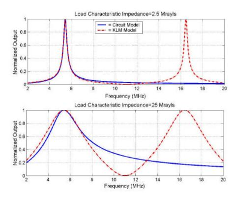
Figure 5.2: Comparison of output simulation results from the RLC circuit model and the KLM model under two different load conditions.
