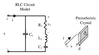
Figure 5.1: Equivalent RLC circuit model for a piezoelectric transducer.
