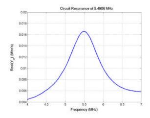
Figure 5.3: Example measured admittance curve for one of the transducers.
