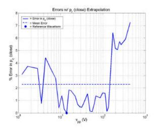
Figure 5.4: Typical errors in  $p_c$  using  $p_r$  as an extrapolation factor.
