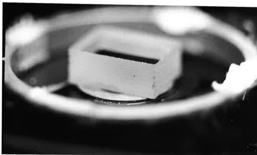
c) close-up of spacer and coverslip on the microscope slide
